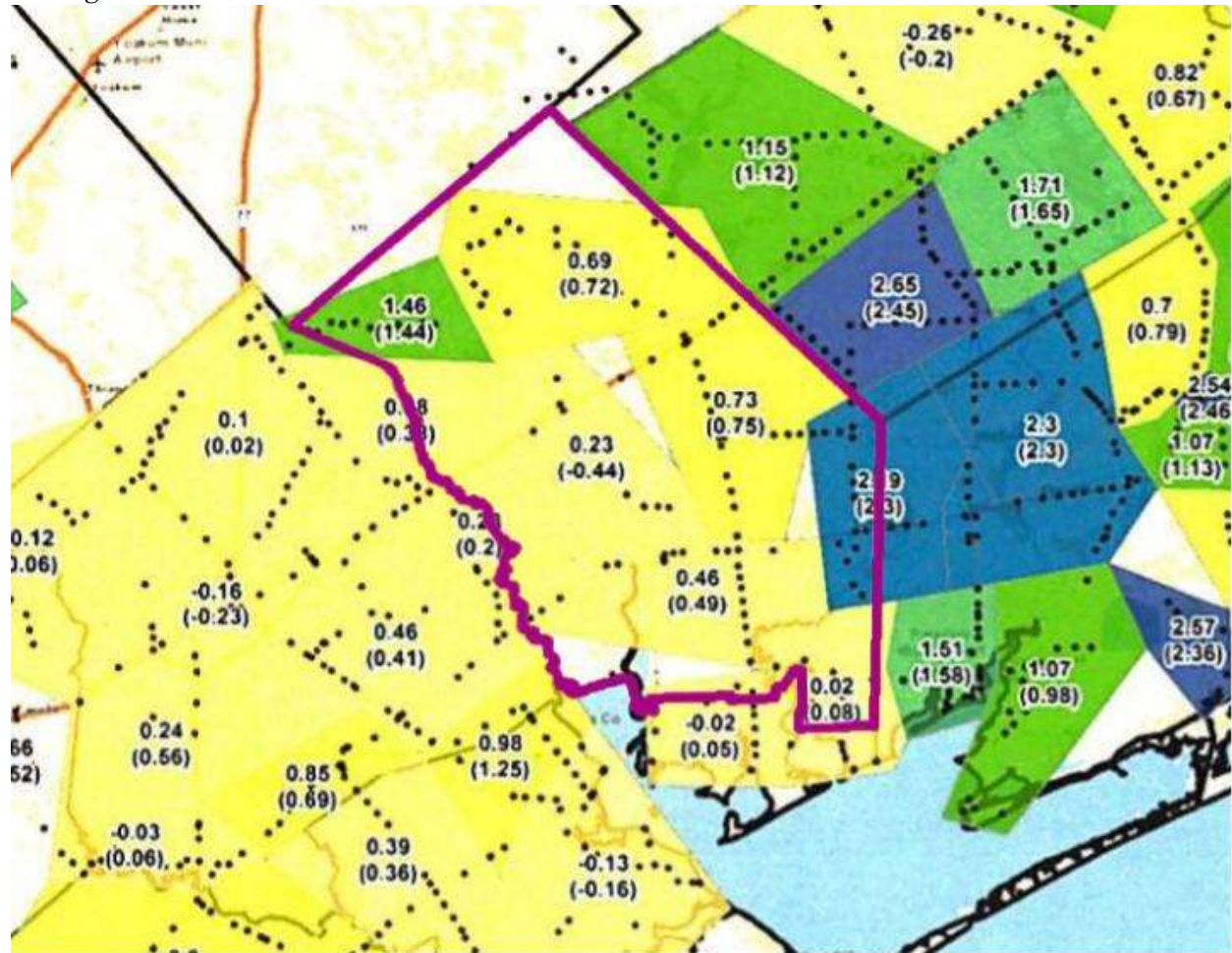
Figure 20-2. Estimates of Land Subsidence Rates in Jackson County Based on the Analysis of Remote Sensing Data
